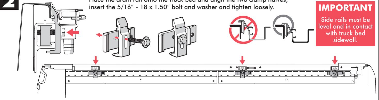
**3** Insert the foam block into the drain rail and use it to position the rail edge 1" from the bed sheet metal. If the truck has a bedliner, the distance will be smaller. **Make sure that both rails are even.**
