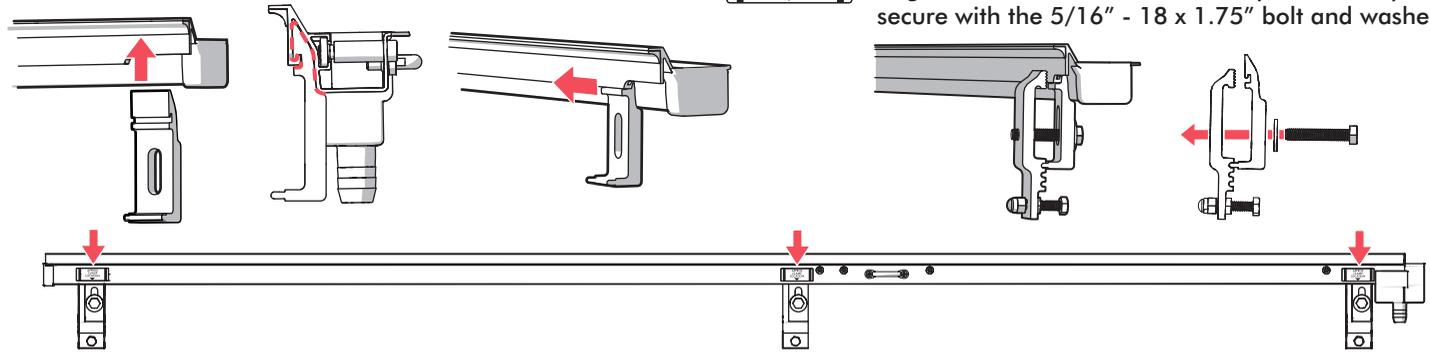
**2** Position the drain rail on the truck bed, insert the foam block into the drain rail and use it to position the rail edge 1" from the bed sheet metal. If the truck has a bedliner, the distance will be smaller. **Make sure that both rails are even.**
